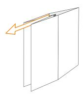
1. Fold out the flatly delivered column material at the glued straps. The object takes on the hexagon shape.
